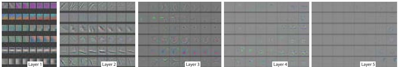
Figure 4. Evolution of a randomly chosen subset of model features through training. Each layer's features are displayed in a different block. Within each block, we show a randomly chosen subset of features at epochs [1,2,5,10,20,30,40,64]. The visualization shows the strongest activation (across all training examples) for a given feature map, projected down to pixel space using our deconvnet approach. Color contrast is artificially enhanced and the figure is best viewed in electronic form.
